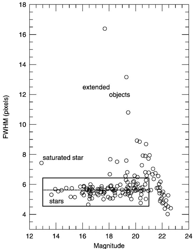
FIG. 6.—Object FWHMs vs. apparent magnitude in a single galaxy field. We use the fact that the FWHM of a star does not depend on its brightness to separate stars and extended objects, as labeled on the plot. For the purpose of our semiautomated seeing measurements, we excluded saturated stars and those that are too faint to yield reliable measurements. The filled box encloses the objects that were used to compute the mean stellar FWHM for this field (dotted horizontal line).
